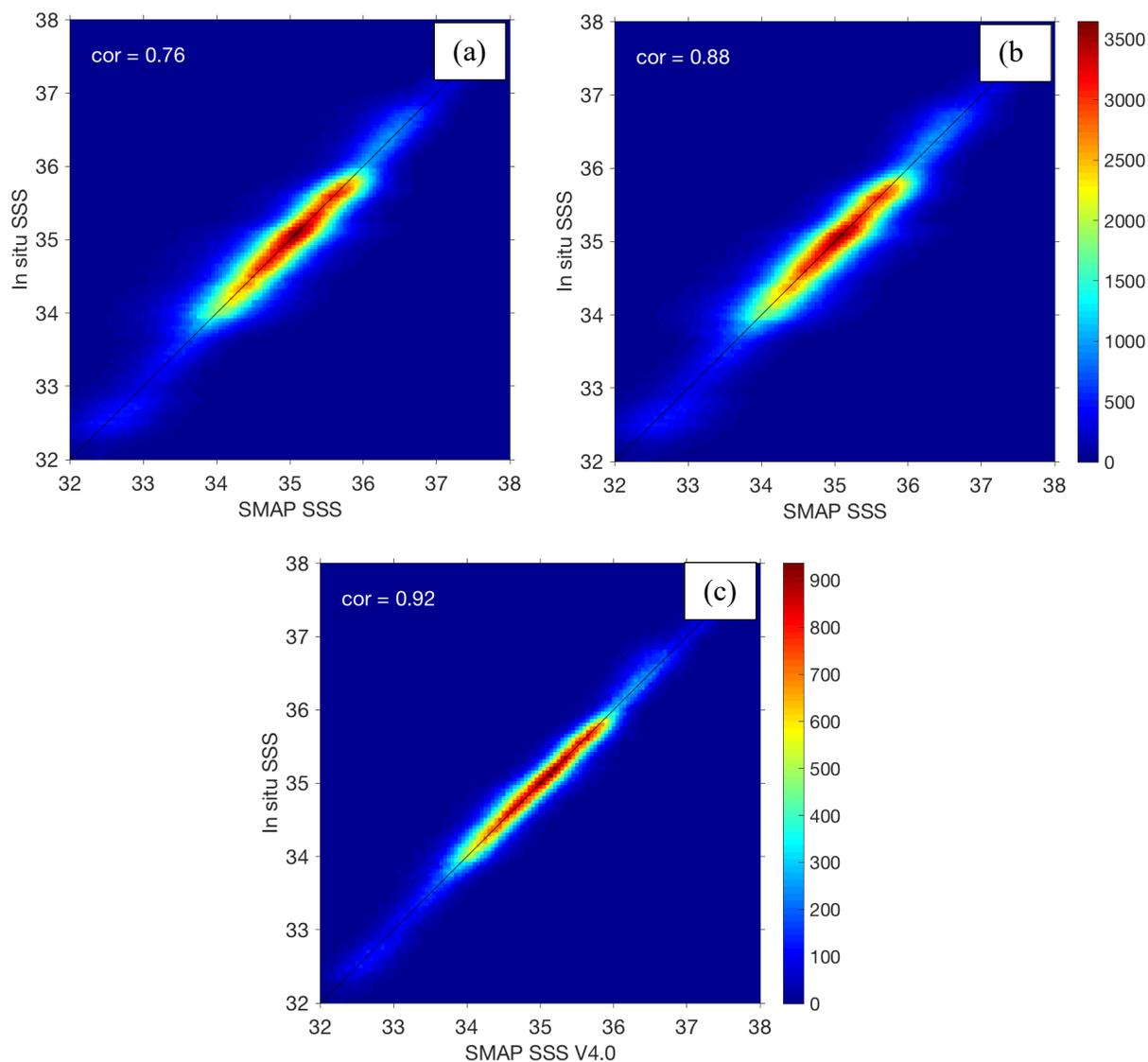
**Figure 14. Scatter plots of SMAP Level-2 (abscissa) and co-located in situ data (ordinate). (a) SMAP V3.0 satellite-centered matchup, (b) SMAP V4.0 satellite-centered matchup and (c) SMAP V4.0 in situ-centered matchup.**
