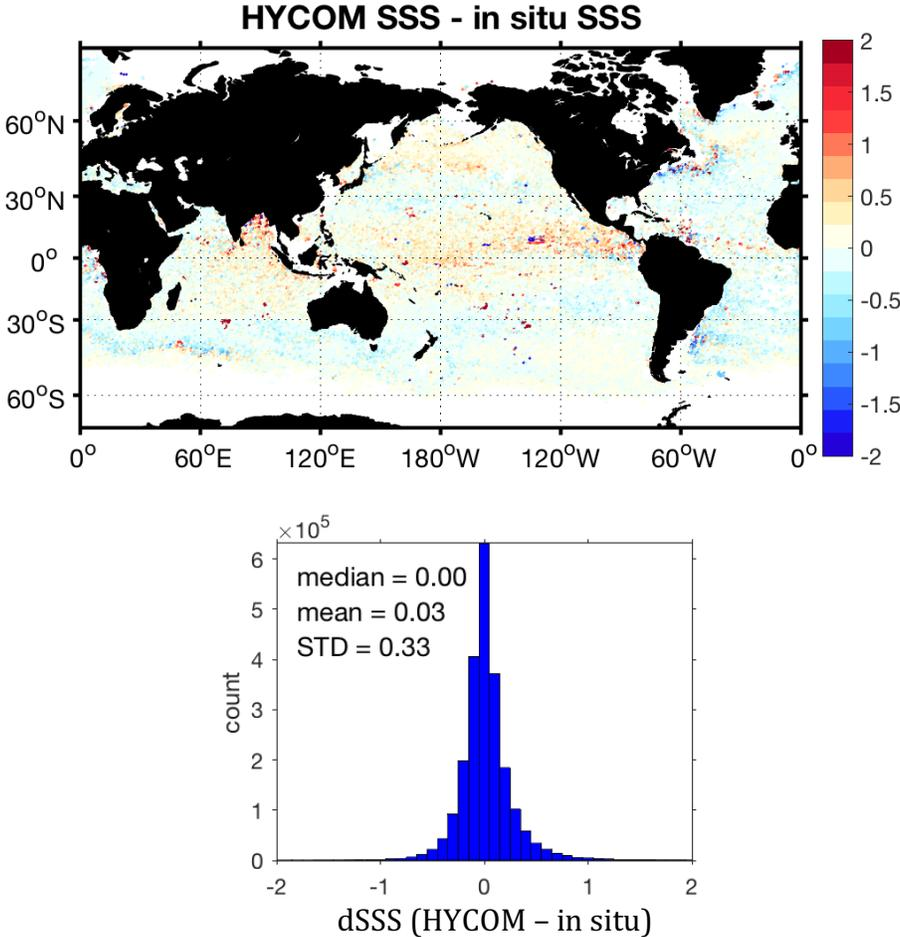
**Figure 4. Salinity differences between co-located HYCOM and in situ.**
