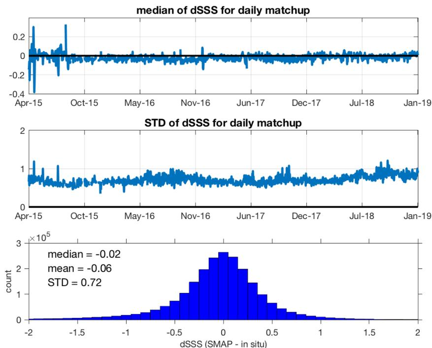
**Figure 11. Statistics of the salinity differences for SMAP V3.0. (a) Time series of daily median of the differences (b) time series of daily STD of the differences and (c) histogram of the differences.**
