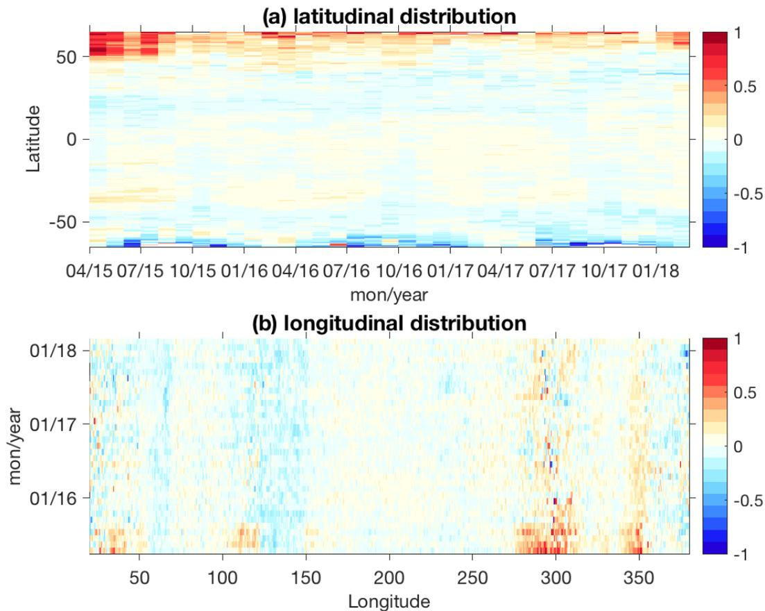
**Figure 16 (a) Latitudinal distribution of zonally averaged and (b) longitudinal distribution of meridional averaged of SMAP - in situ SSS differences.**
