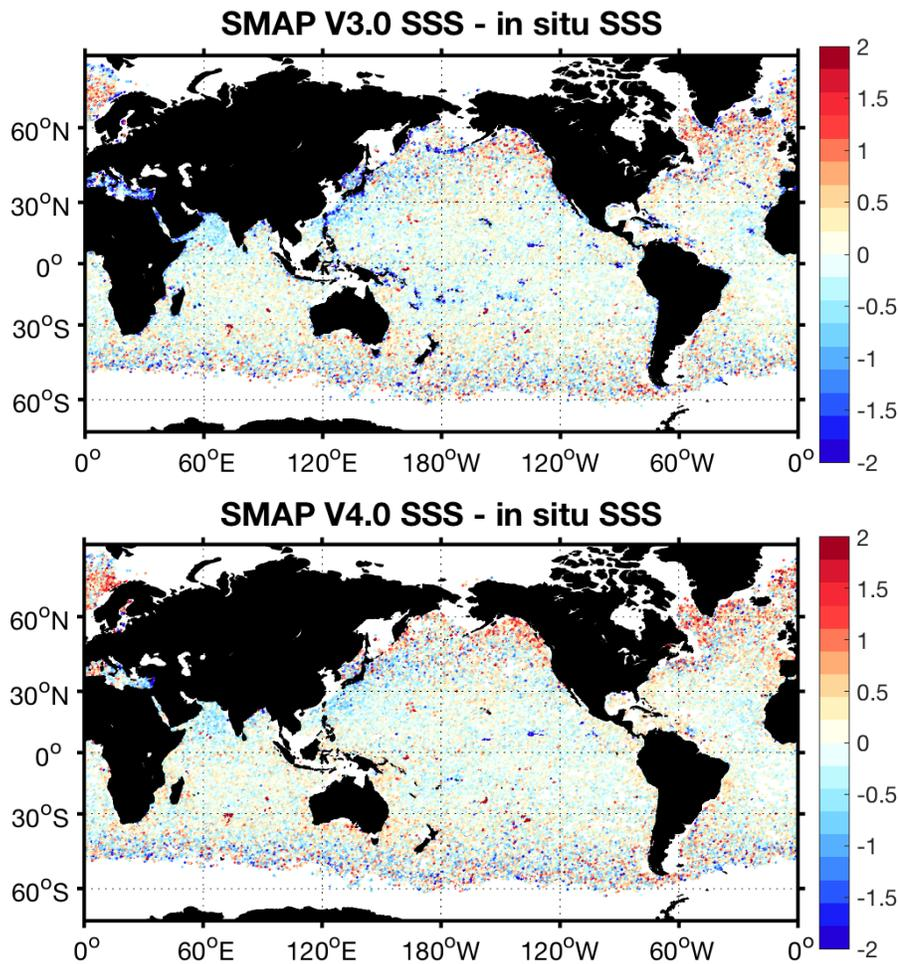
**Figure 2. Global maps of SSS differences defined as the SMAP (a) V3.0 and (b) V4.0 data minus the co-located in situ salinity (satellite-centered).**
