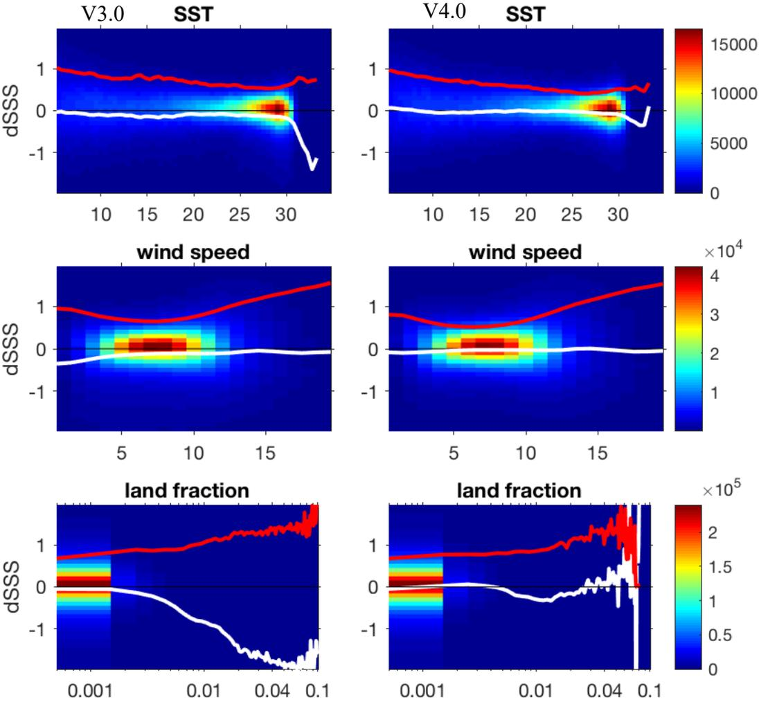
**Figure 7.** Differences of SMAP L2c data and in situ salinity compared with (upper) different sea surface temperature in  $^{\circ}C$  (middle), wind speed in m/s and (bottom) and land fraction in V3.0 (left) and V4.0 (right). White lines show the salinity biases and red line shows the standard deviation.
